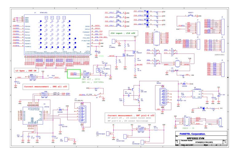
Evaluation board can be used as a reference design for using modules. EV BT840F V4 is designed for the BT840F soldering pads with 61 pins. These 21 pins in solid dark color are for BT840F.
